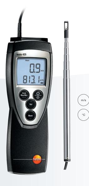
testo 425 is a compact anamometer with a fixed thermal flow velocity probe. The probe head has a diameter of 7.5 mm. With the extendable telescope (length max. 820 mm), the measuring instrument is suitable for flow velocity measurement in ducts. The testo 425 also measures extremely accurately in the low flow velocity range. The volume flow is directly shown in the display. For the purposes of volume flow calculation, the duct area can be
