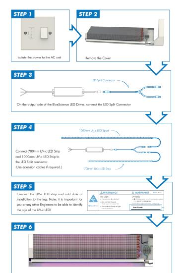
Lay the UV-c LED Strip on the top of the drip tray, making sure the UV-c LED's are facing in towards the unit. UV-c LED's must not radiate out or point out in the direction of the room.
